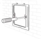
5. Slant the switch plate cover and put it in place, then secure the plate cover to the switch from the bottom with a KM2 screw.
